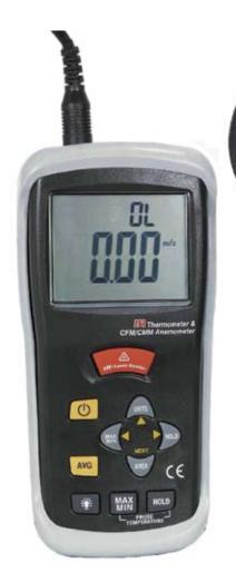
Model 12844 CFM/CMM Anemometer measures Air Velocity, Air Flow (Cubic Feet per Minute [CFM] & Cubic Meters per Minute [CMM]) and Temperature. Temperature is measured with a probe in the vane or a non-contact InfraRed senosor with laser targeting. The 12844 has memory for 8 area values and 20 average values for Max/Min.
