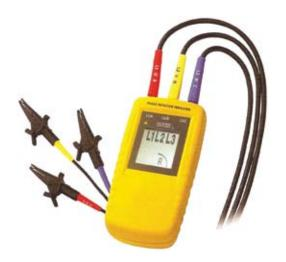
Model 12701 Phase Rotation Indicator detects the rotary field of three phase systems. Features 3 phase indication, indication of phase rotation and clear LCD display. No battery is required. Includes manual and soft case.
