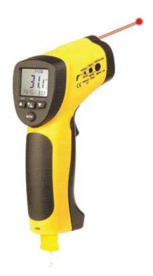
Model 16505 InfraRed and K-probeThermometer is ideal for temperature measurement of hard to reach areas and materials. Built-in laser pointer focuses the target for high accuracy measurements and a type-k probe allows for dual measurement. Features 20-point memory, compact, guntype design and includes manual, battery, k-probe and soft case.
